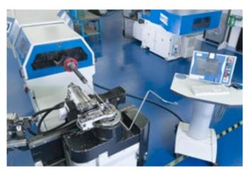
Using different bending procedures and techniques, the ultra-modern 10-axis bending centres and our many years of experience enable us to implement virtually all bending geometries, and that includes the bending of internally electropolished stainless steel tubes.
