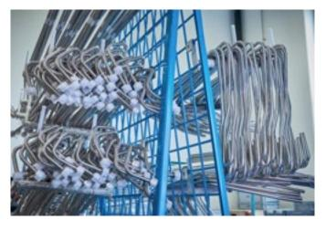
The tubes are bent and assembled in economical lot sizes. Delivery is made on time and in the agreed quantities directly to the customer, and can be incorporated in the production cycle there.
