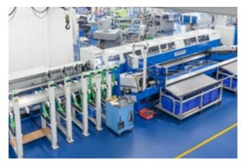
Modern, fully automatic tube saw for up to 3,000 cuts per hour with accuracy of  $\pm\,0.2~\text{mm}.$
